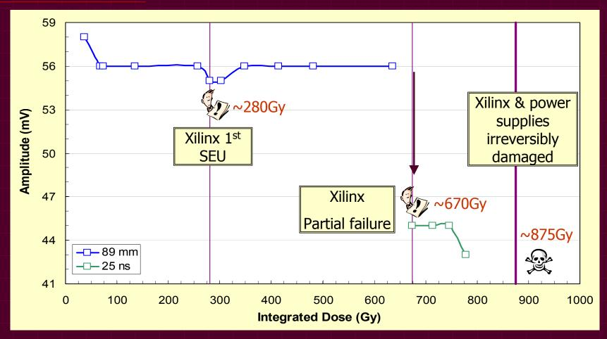
Note: Measures at lab. show no amplitude or offset change appreciable so no efficiency loss or threshold current increase is appreciable up to ~875Gy.
