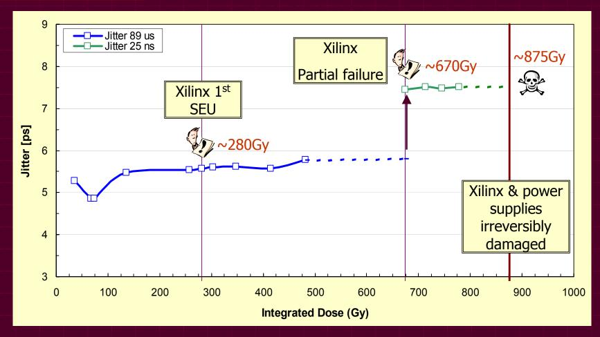
Note: After 2 weeks of annealing, new measures at lab. were done:  $89\mu s \rightarrow 5.4ps$ ,  $25ns \rightarrow 5.4ps$
