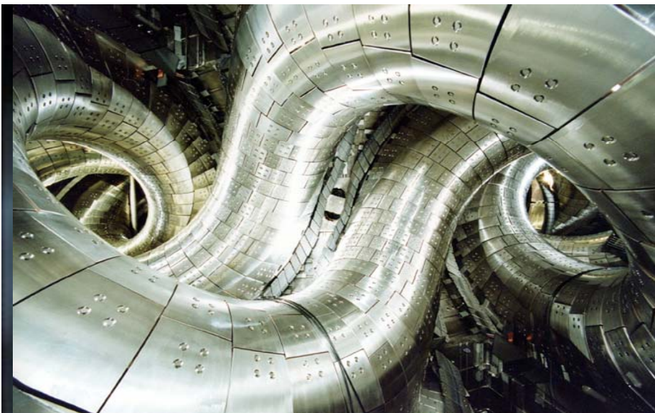
LHD: R= 3.6, 3.75, 3.9 m; a= 0.6-0.65 m M=10, l=2, n=1, m=1 island in the edge.
