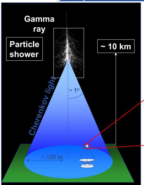
Cherenkov light Image of particle shower in telescope camera
