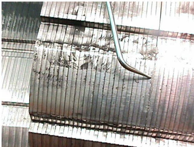
Damage caused by a short circuit developed during a quench in a LHC dipole prototype
