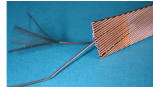
Superconducting cable made of strands
