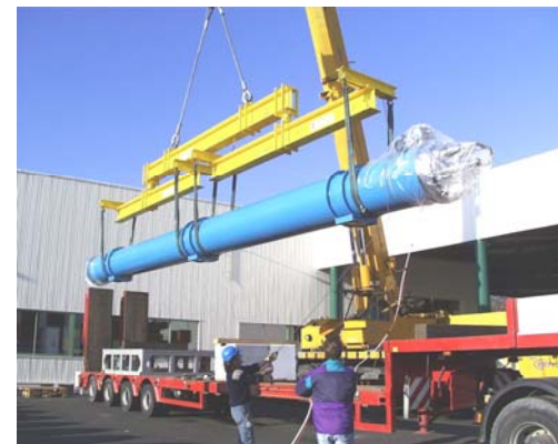
A 15m truck unloading a 27 tons LHC dipole
